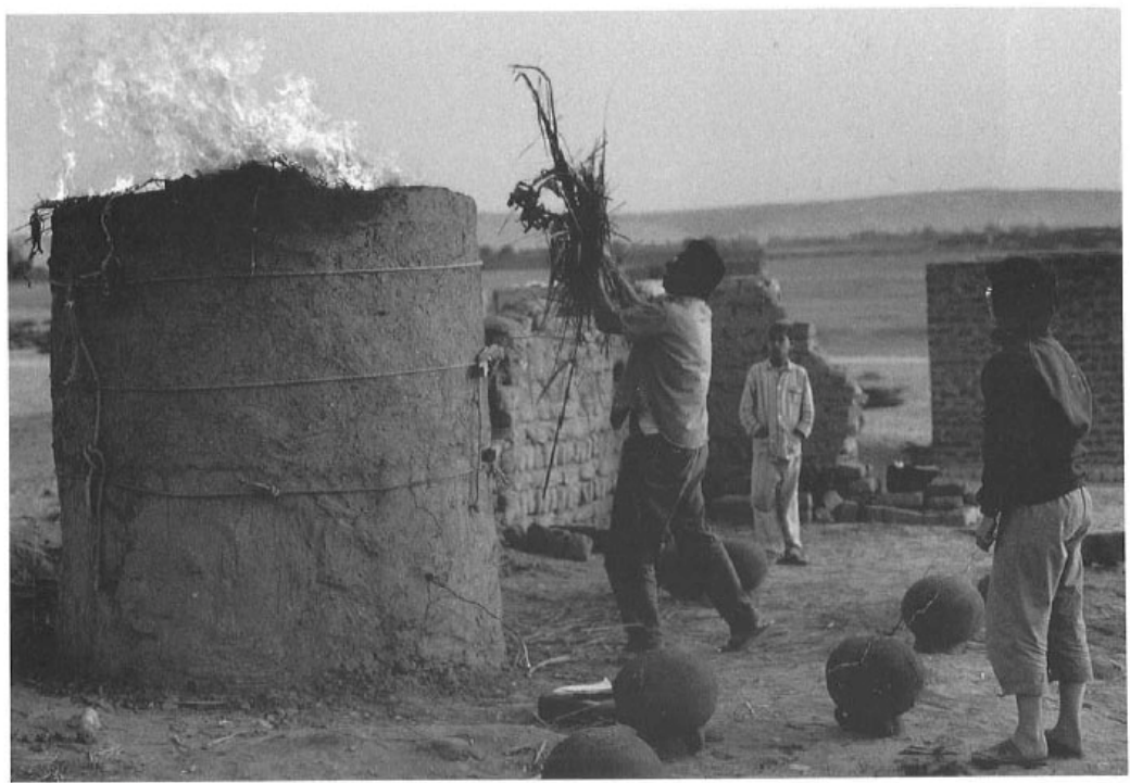
Figure 8.17. Throwing clean fuel onto the kiln top in order to decarbonise it. This marks the final stage in the firing of the kiln.
