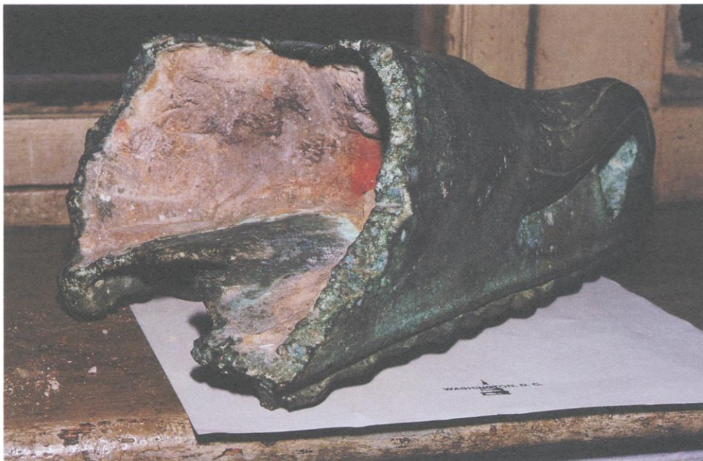
FIG. 3. Serpent head from the Delphi Tripod, in the Archeological Museum, Istanbul. View of core material with red iron oxide remains of armature. The bronze casting varies greatly in thickness.
