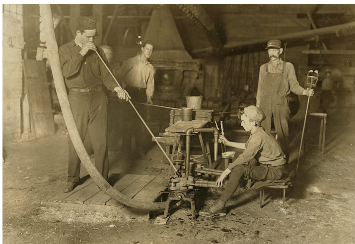
Image 1. A skilled glass blower injects molten glass into a mold assisted by workshop crew. http://www.sha.org/bottle/Glassmaking/gafferandmoldboy.jpg
